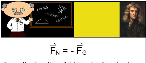
The normal force is equal in magnitude but opposite in direction to the force of gravity. It occurs when an object comes in contact with any surface and always acts perpendicularly to that surface.
