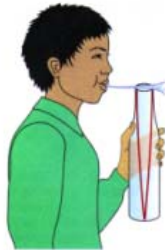
▲ Figure 8.32 The tone produced when you blow across the top of an open bottle depends on the length of the air column.
